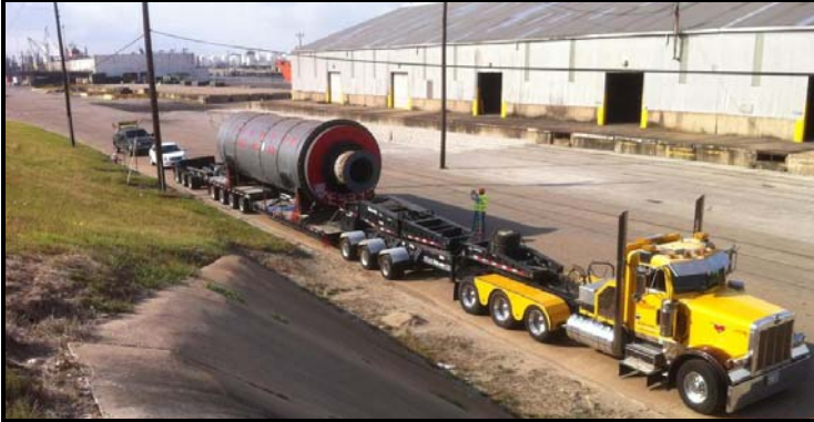
Brian Johanson (908281) hauled a Ball Mill from Houston, TX to Fort Smith, AR. Dimensions were 145'L x 12'W x 15'H, 261,000 pounds.
