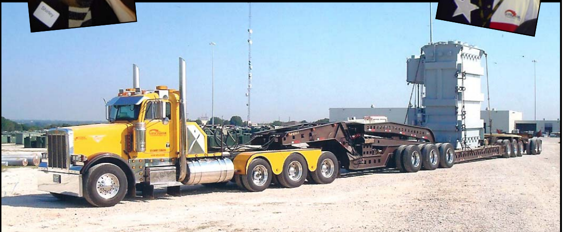
Brian Johanson (908281) moved this TXU transformer to Lancaster, Texas. Dimensions were 117' L x 10'6" w x 19'8"l.
