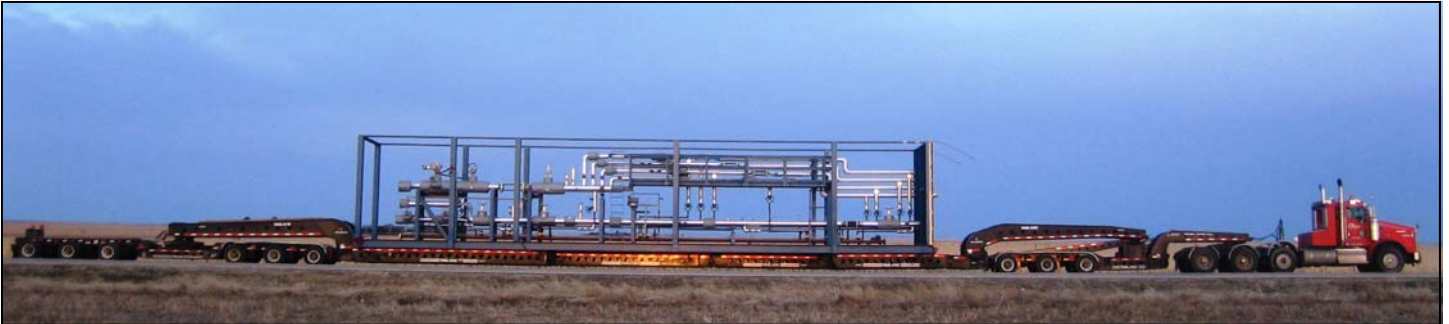
This steam skid was moved from Locust Grove, OK to Nisku, AB, Canada by Howard Broussard (900247) . Dimensions were 181'6" L x 12' W x 16'6" H.
