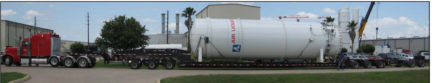
This liquid nitrogen tank moved from Houston, Texas to Indianapolis, Indiana by Kervin Clark (900120) . Dimensions were 144'L x 13' W x 15'8" H.
